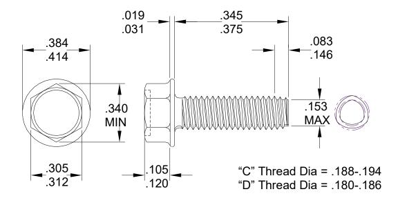
Unspecified and Performance Standard: ASME B18.6.3 Material: Carbon Steel Heat Treat: Case Hardened Rc45 Min, Core Hardened Rc28-38. Finish: LIGHT PHOS/ 1 BASECOAT-DP KL100/ AND 1 COAT DELTA SEAL SILVER PER ACGO SPEC# 705100300 SST 96 Hr White, 240Hr Red
